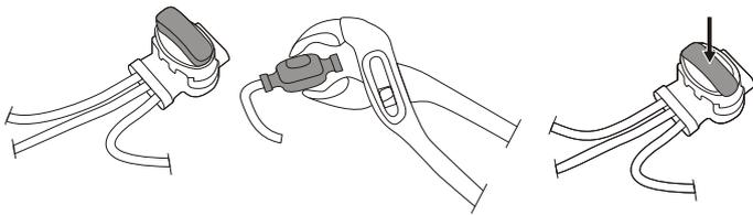
Insert both ends of the boundary wire as well as the end of the guide wire into the splice and guide wire connector. Check that the wires are fully inserted into the splice and guide wire connector so that the ends are visible through the splice and guide wire connector.
